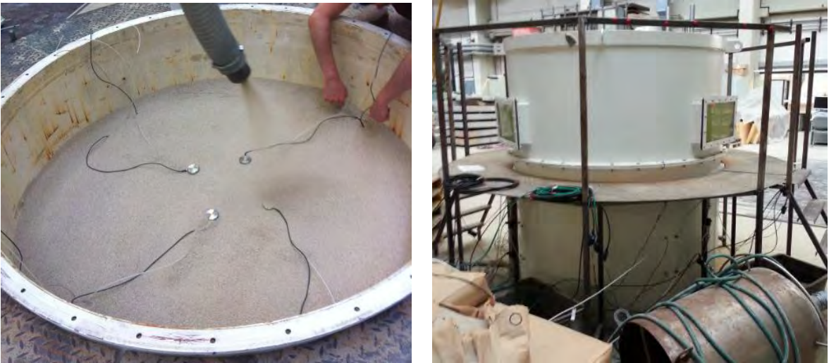
Figure 2-14 Disposition of the load cells in the left; Container in the right.
