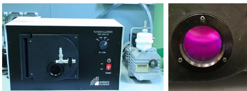
Figure 2.7 Plasma treatment: (a) plasma Cleaner by Harrick Plasma used in BIAMET Laboratory; (b) color of plasma when an adequate quantity of oxygen is present in the chamber.
