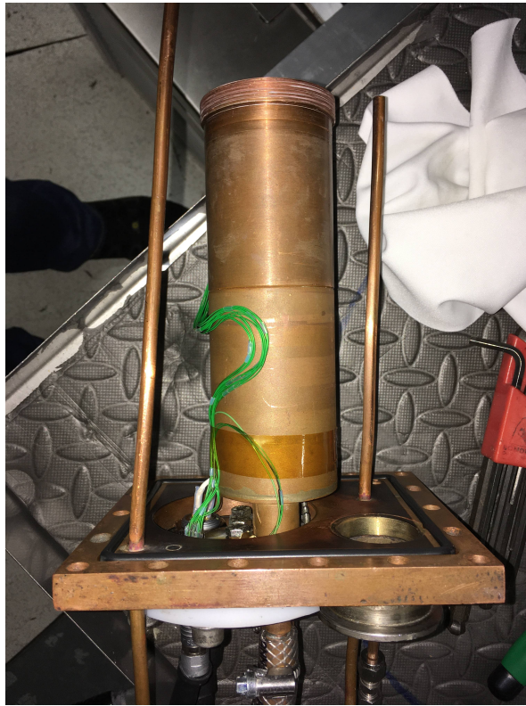
Figure 14: The calorimeter system installed at the end of the target chamber in February 2020. The hot side is on the top in the picture, the two copper tubing on the sides are connected to pressure gauges.
