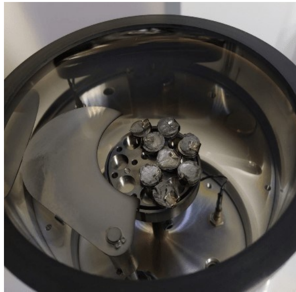
Figure 2.8. Freeze-dried hydrogel samples preparation before SEM images acquisition: gold and palladium sputtering under vacuum.
