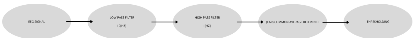
(c) Pre-processing pipeline with eye blinking removal: two Butterworth filters, CAR, and a threshold
