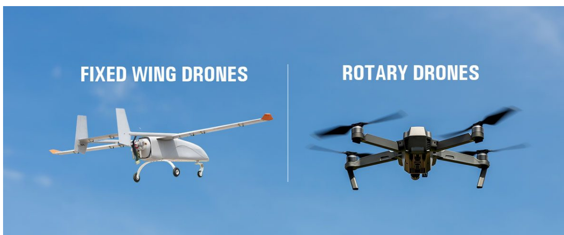
Figure 1.10: Comparison of UAV Types: Rotary-wing UAVs offer vertical and short take-off and landing, hovering, and omnidirectional flight with easy maneuverability. Fixed-wing UAVs, characterized by rigid wings, provide forward lift, have a simpler structure, longer flight range, and lower maintenance and repair costs.
