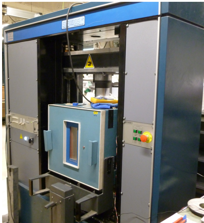
Figure 4.4: Instron testing machine TT-D1115.
