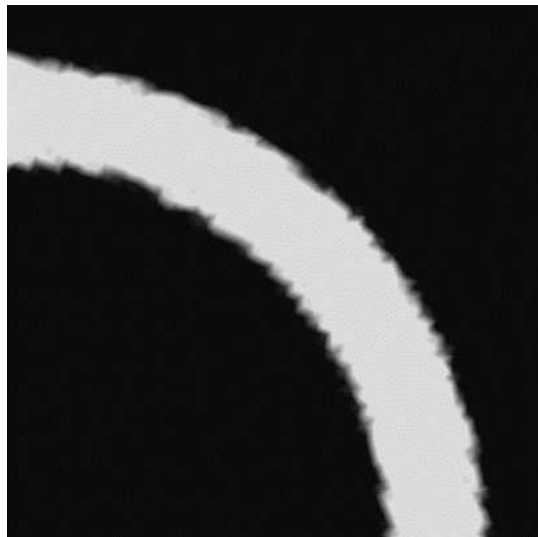
Figure 4.3: Example of the checkerboard pattern caused by the size of the mesh elements. Manufacture however is not constrained by the size of a mesh, and therefore a result with borders as smooth as possible is to be preferred.
