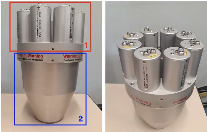
Figure 3.5: Photo of a BGO anti-Compton shield of GALILEO. Left: 1. Photomultiplier Tubes; 2. Bismuth Germanate Crystals. Right: view of the eight BGOs. Figure taken from Reference [30].
