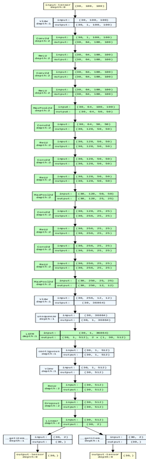
Figure A.3: Simplified VGG architecture with normal convolution and LSTM module.
