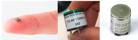
Figure 3.7: Examples of low-cost chemical sensors. (From left to right) MOX sensor (Model: Figaro TGS 8100); AGS sensor (Model: Alphasense CO-AF); PID (Model: RAE Systems PID 10.6 eV) [28].
