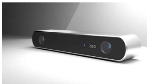
Figura 4.1: Stereo camera ZED [23]
