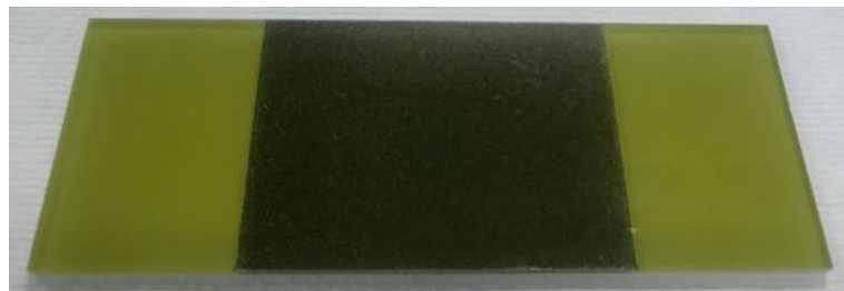
Figure 7.5: Speckle pattern applied using a film on a finished specimen with the underside painted in matt white.
