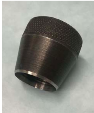
Figure 5.3: Mould for cutting the PTFE inserts.
