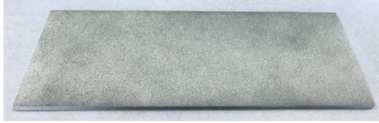
Figure 7.3: Speckle pattern applied using aerosol cans on a finished specimen.
