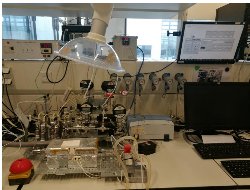
Figure 2.2: View of the laboratory experimental setup for catalytic activity tests.
