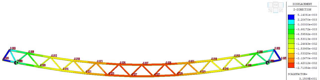
Figure 3.21. Deflection of bridge in Midas
