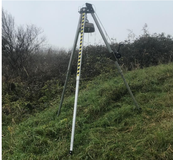
Figure 12: The weight drop. an active seismic source in the Porto Tolle project.
