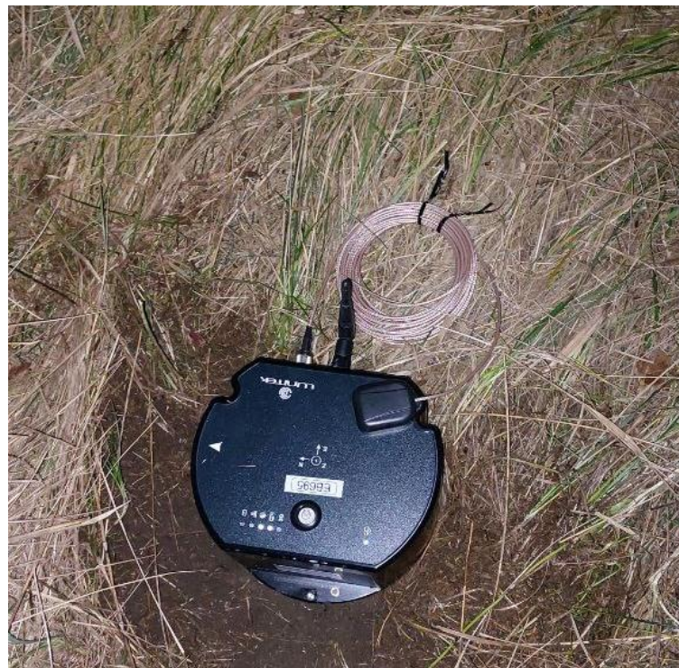
Figure 14: Lunitec velocimeter installed in the field of acquisition in Porto Tolle.
