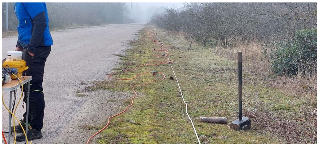
Figure 11: One of the geophone array lines in the Porto Tolle project, including the sledge hammer as the source of the MASW data acquisition.
