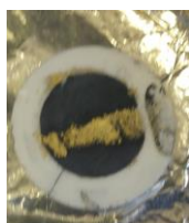
Figure 32 Gold paste on LSCM electrode is easily removed. A good contact is not achieved.
