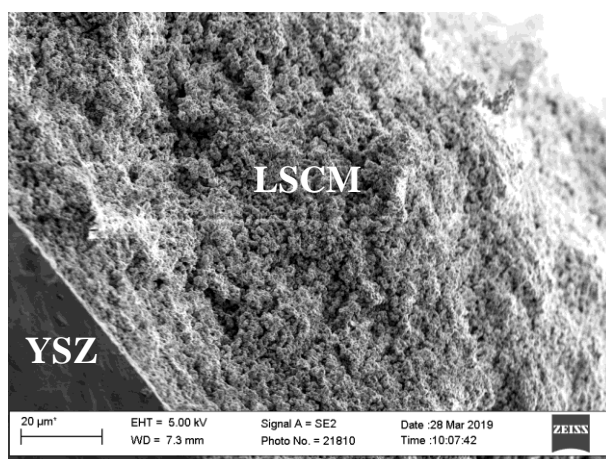
Figure 30. Full cell view taken by SEM, 5.00kV and 2k of magnification. YSZ dense electrolyte (black) and porous electrode layers.
