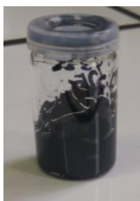
Figure 26 Photo of LSCM ink deposited inside a vial before its tape casting over electrolyte pellets.
