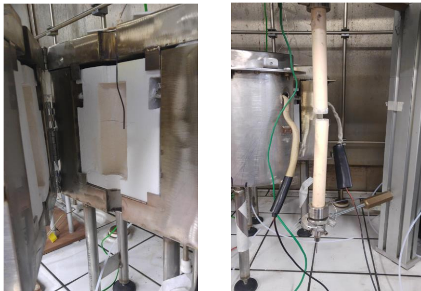
Figure 27. Images of the experimental setup. On the left, there is the oven inside which measurements take place, it is also visible one of the thermocouples used in the apparatus. On the right, the two alumina tubes are presented.
