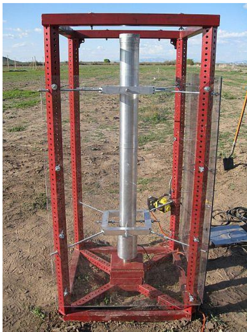
Figure 1.19 - Vertical test with nozzle pointing up (team Daedalus from Arizona State University) [8].
