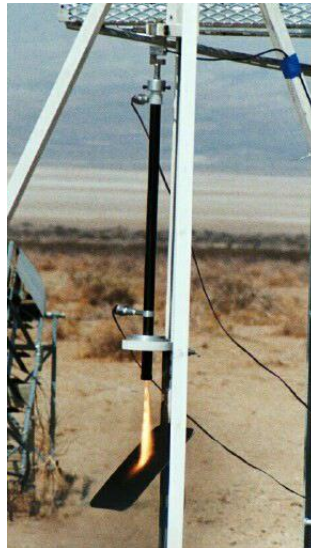
Figure 1.18 - RATTworks L1000 motor tested vertically with nozzle pointing down [7].
