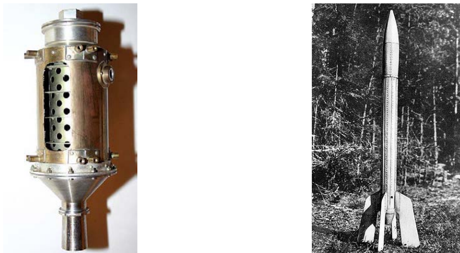
Figure 1.6 - GIRD 09 combustion chamber (left) and complete rocket (right).
