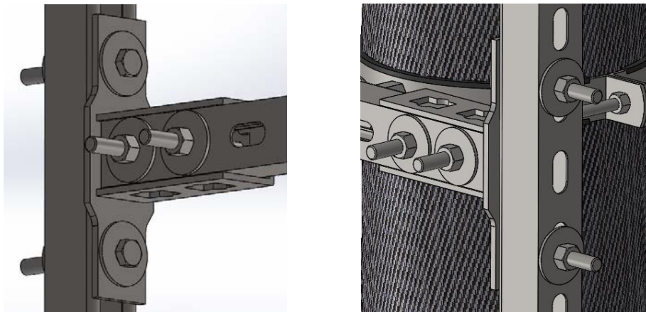
Figure 4.17 - Saddle bracket junction.
