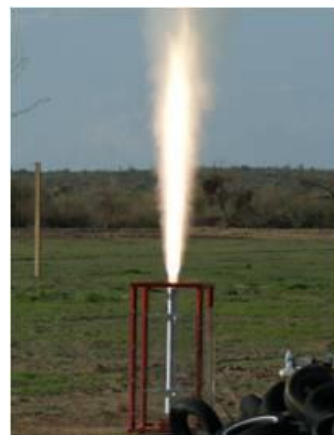
Figure 1.19 - Vertical test with nozzle pointing up (team Daedalus from Arizona State University) [8].
