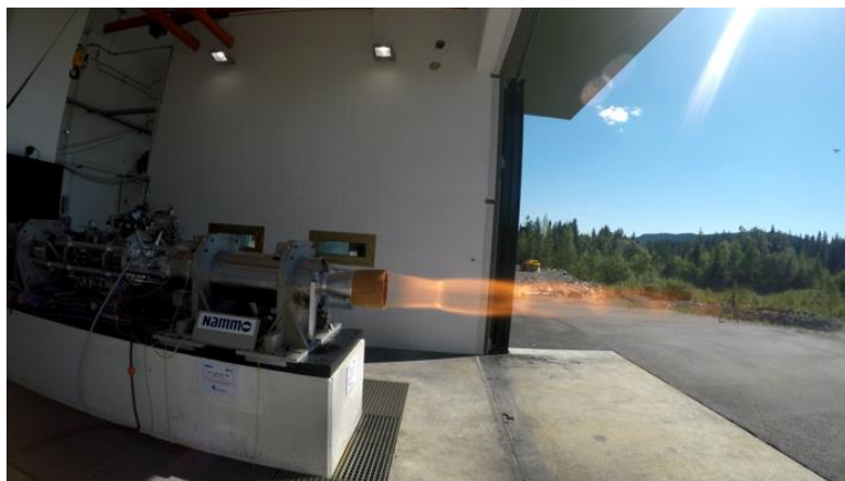
Figure 1.17 - Nammo Nucleus tested horizontally [6].
