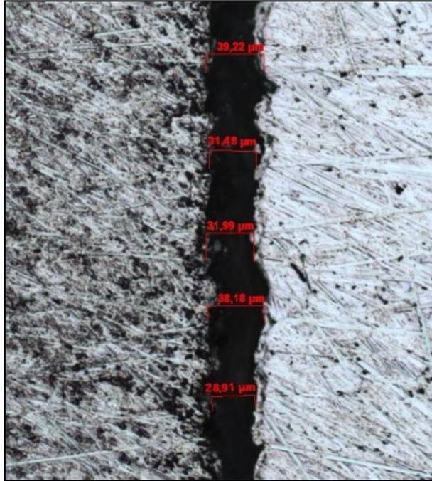
**Fig. 5.9: Crevice between AM50 HP (on the left) and EN AW 6083 (on the right), sample number 2 – optical microscope 200x.**
