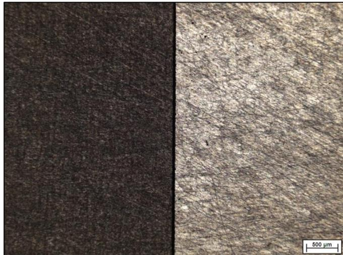
**Fig. 5.8: Crevice between 1 cm x 1 cm square of magnesium AM50 HP and 1 cm x 1 cm square of aluminum EN AW 6083 – optical microscope 25x.**
