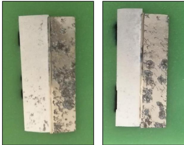
**Fig. 6.21:** Samples aluminum + magnesium after 100 the immersion tests: (right): 6 days of diffusion, more visible signs of corrosion on aluminum, (left) 7 days of diffusion; in both couples, magnesium is on the left.
