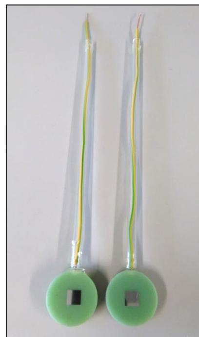
**Fig. 5.5:** An example of two samples used for the corrosion test: material embedded in the epoxy and connected to the wire.
