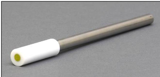
**Fig. 5.3: Working electrode with the circular active area exposed.**
