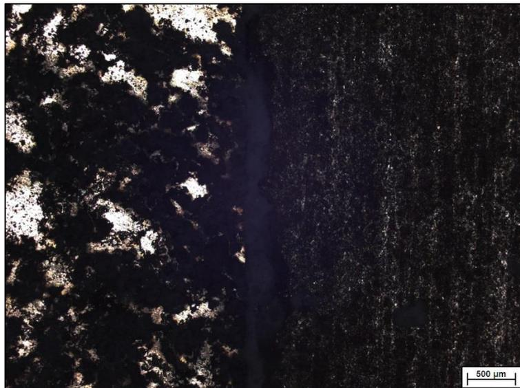
**Fig. 6.4:** Border between AM50 HP and EN AW 6082 with a lot of corrosion products – optical microscope 25x.
