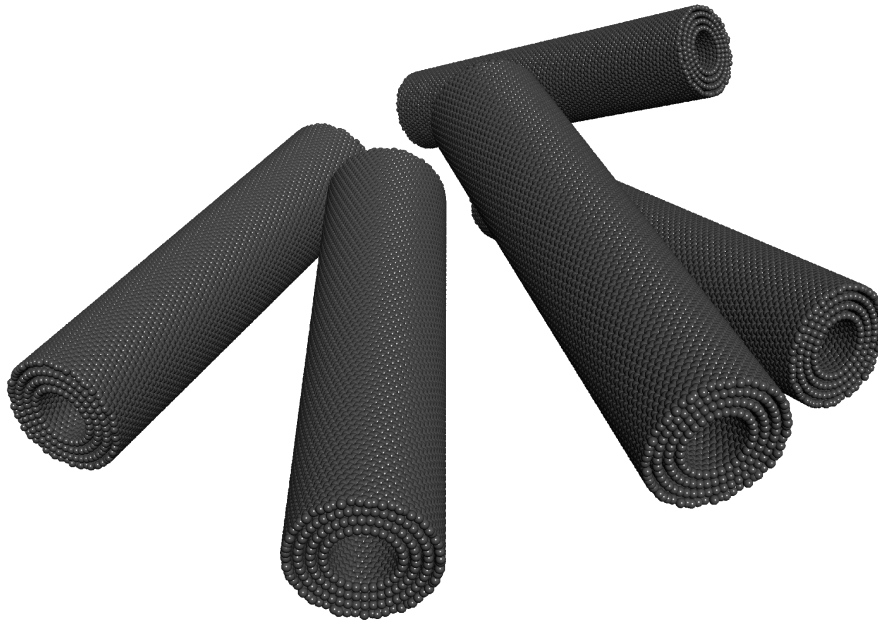
Figure 8: schematic representation of MWCNT structure
