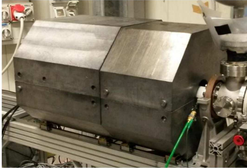
Figure 4.5. The lead shielding around the detectors
