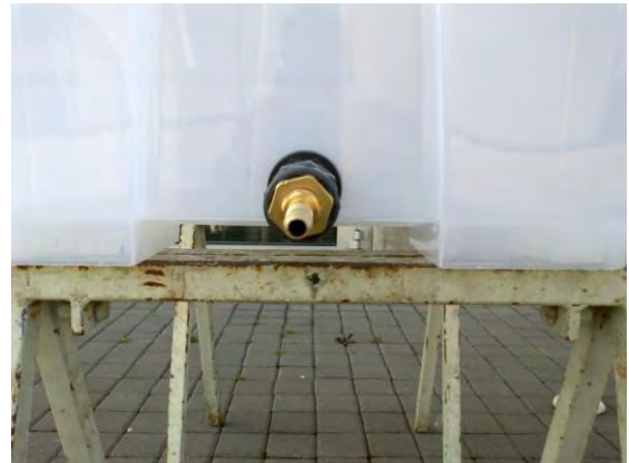
Figure 16. Tap system installed on horizontal subsurface flow tanks
