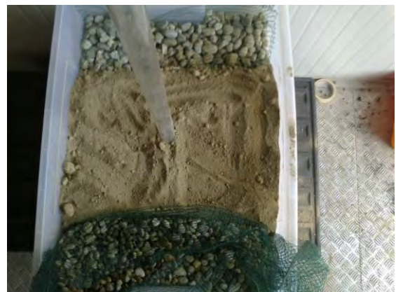
Figure 18. Vertical plastic cylinder inserted in central layer
