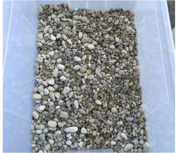
Figure 8. Gravel drainage layer on the bottom of vertical flow tanks
