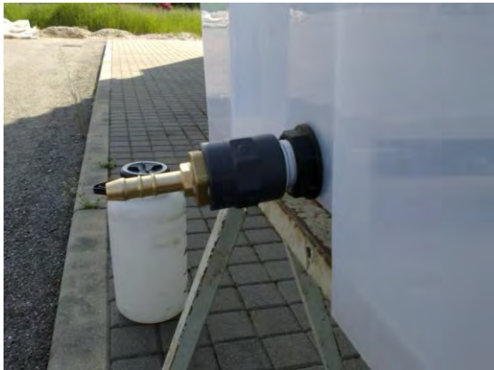
Figure 9. Tap system used to drain effluent water
