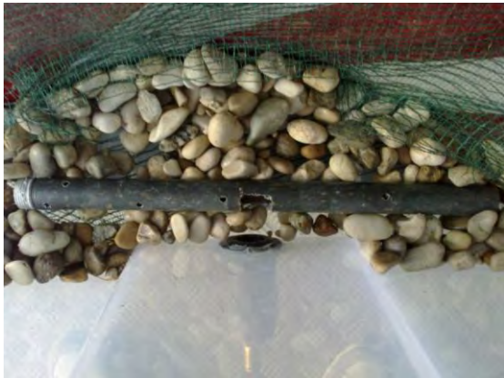
Figure 15. Holed PVC pipe, transversal to the flow pattern, used to promote the drainage of the effluent
