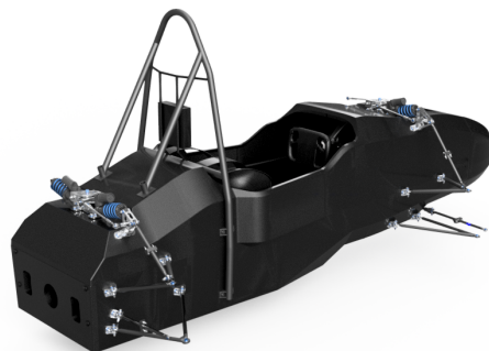
Figure 3.1: Render of monocoque used in the season 2020/2021
