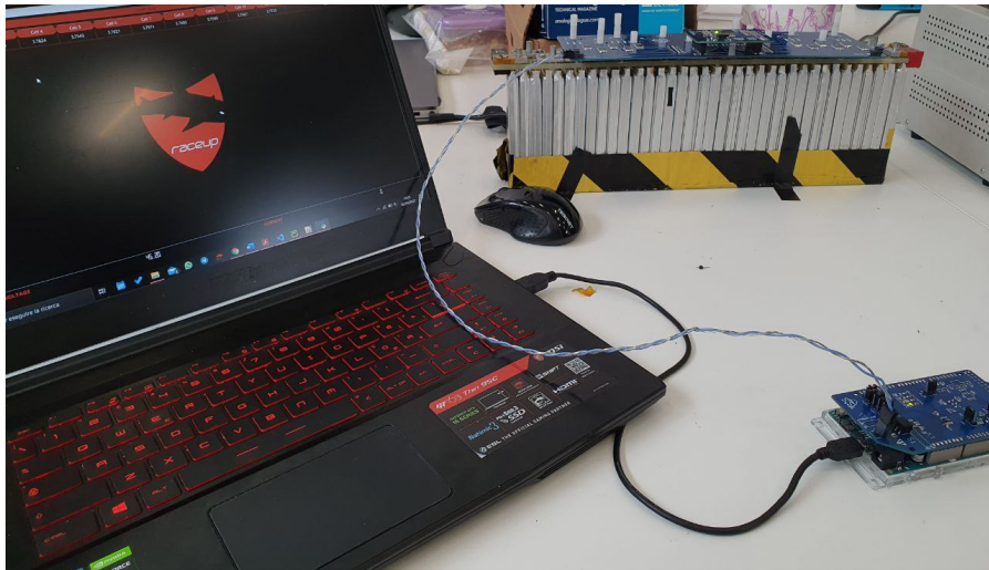
Figure 5.8: BMS System communication test on battery segment
