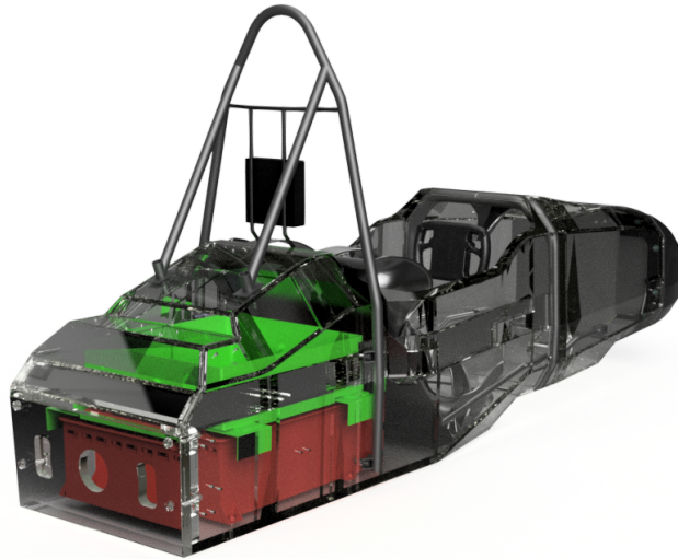
Figure 3.8: Location of the inverter and the tractive system battery in the car
