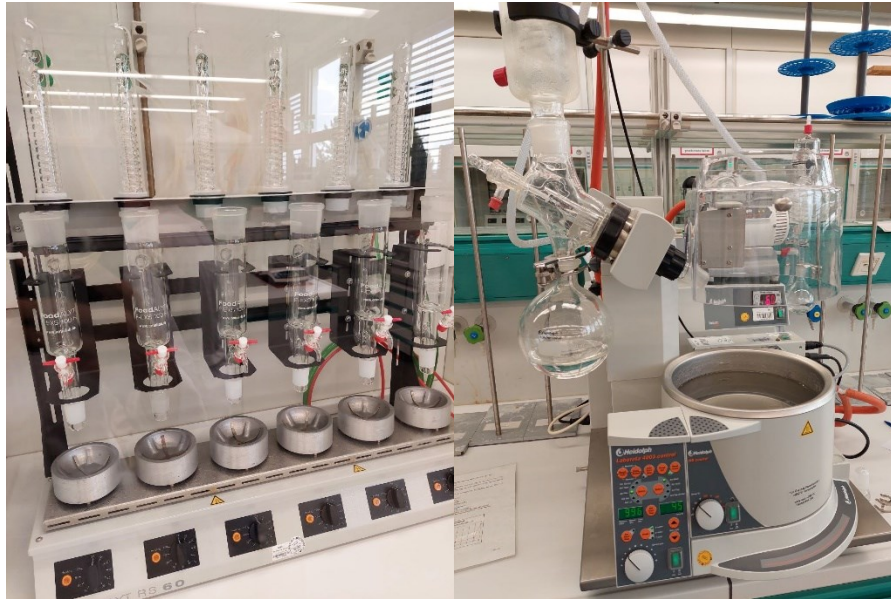
Fig.2 Soxhlet extraction apparatus
