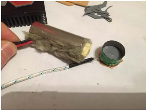
(c) The directional heating can, made from another cell's can and some mineral wool
