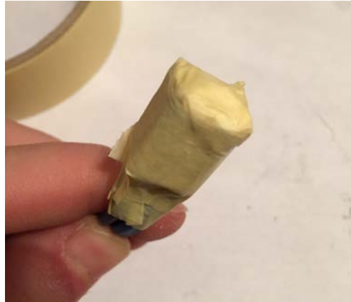
(b) Resistors spreaded in thermal paste and taped, to provide electrical isolation from the case and prevent interferences with the measure
