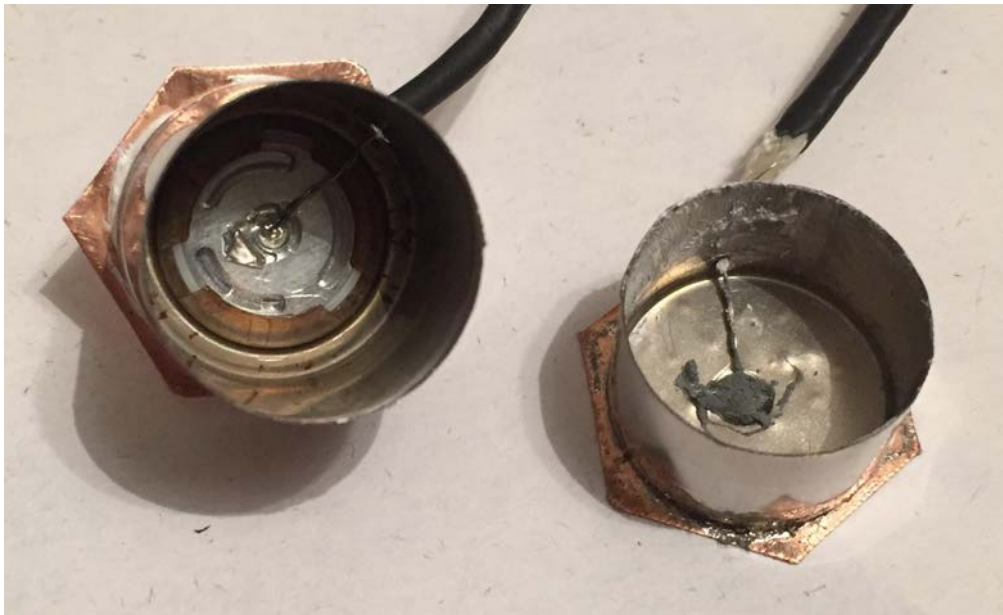
Figure 5.4: Positive (left) and negative (right) tabs, welded to the 0.2mm copper plate and with the K-thermocouple glued in position
