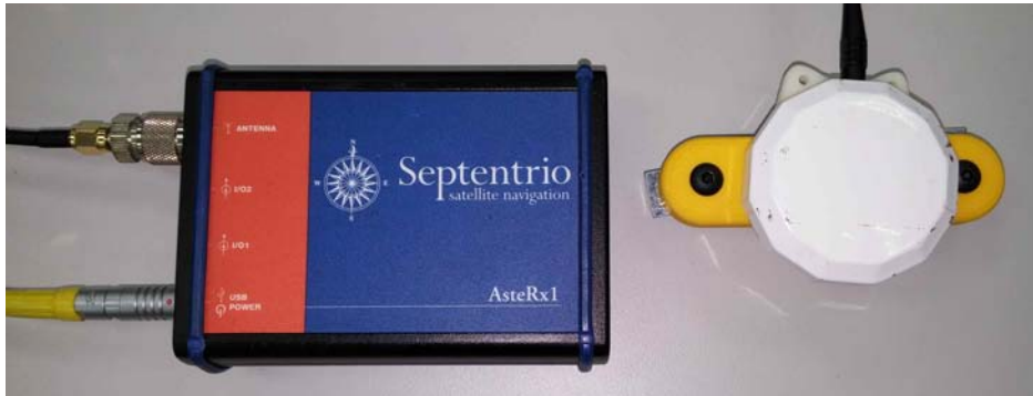
Figure 4.5: Septentrio AsteRx1 GPS/Galileo single-frequency receiver. On the left there is the receiver device and on the right the external antenna.
