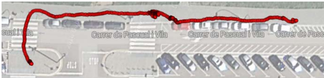
Figure 4.8: GPS fixes produced directly by AsteRx1 receiver.
