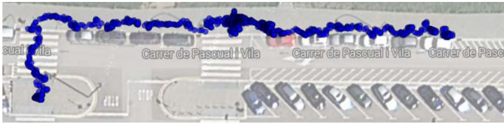
Figure 4.7: GPS fixes produced from raw GPS measurements by raw_gps_ros 's nodes.
