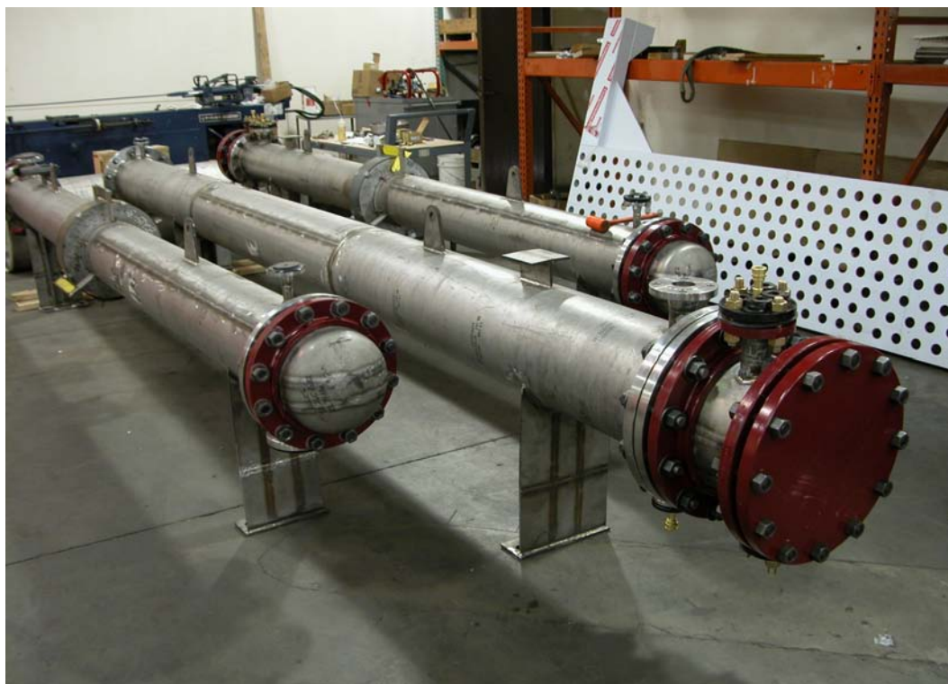
Fig. 7 Standard duplex 2205 Heat Exchanger pipe
