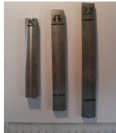
Fig 10. Samples after different cold rolled deformation
