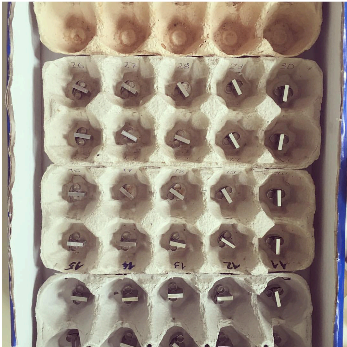
Fig 22. Specimens put in supports and ready for corrosion test
