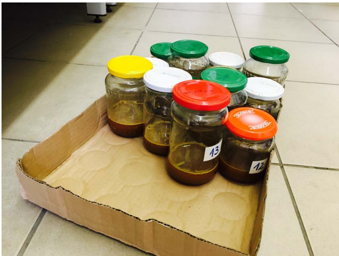
Fig 23. Samples in ferric chloride solution into glass container
