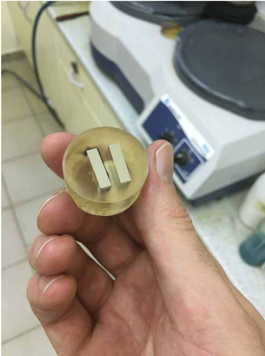
Fig 12. Final result after grinding and polishing
