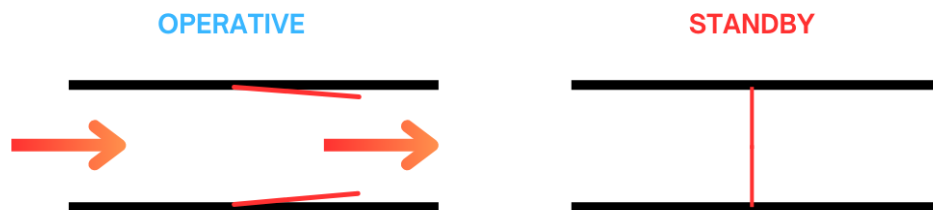
Figure 5.48: Flaps position depending on the different states of the VRFB
