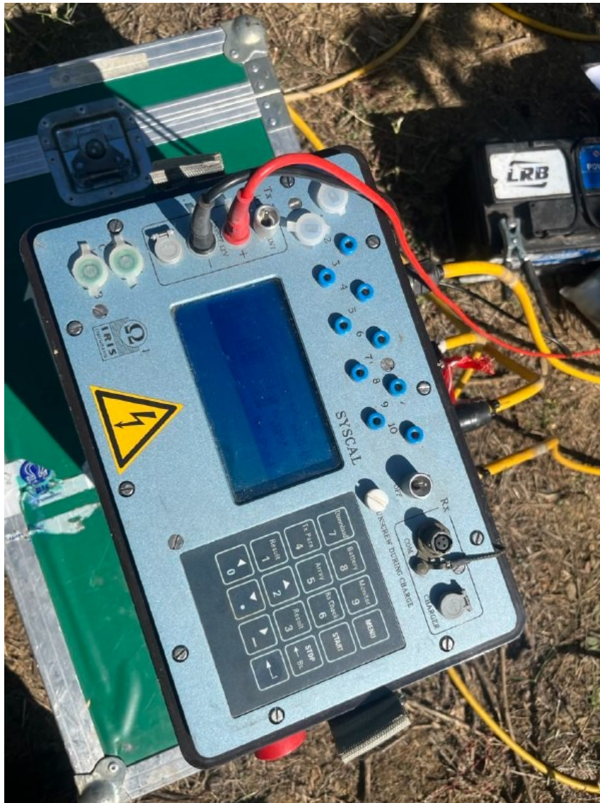
Figure 5.9. SYSCAL PRO Resistivity meter
