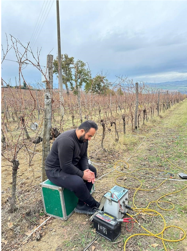
Figure 6.6. Data acquisition with syscal pro georesistivimeter
