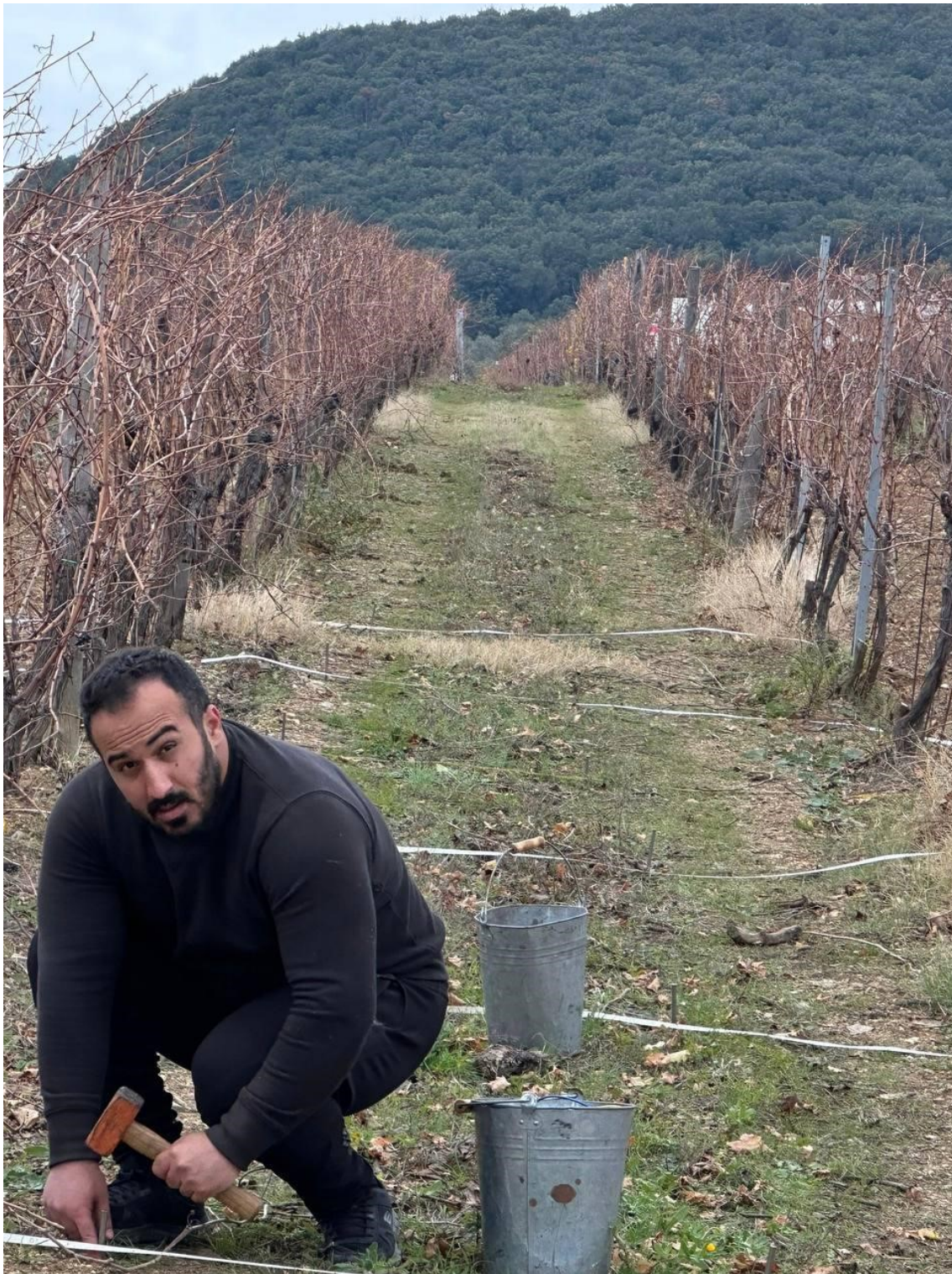
Figure 6.3. putting electrodes with 1m spacing
