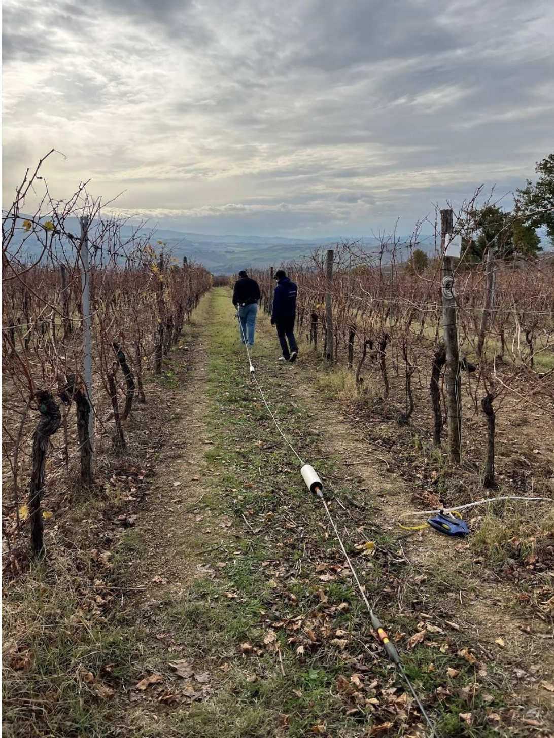
Figure 6.12. OHM mapper Data measurement
