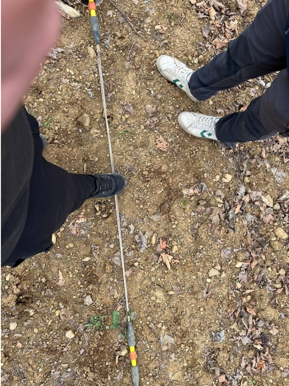
Figure 6.11. ohm mapper measurement with 1.25m non-conductive rope.
