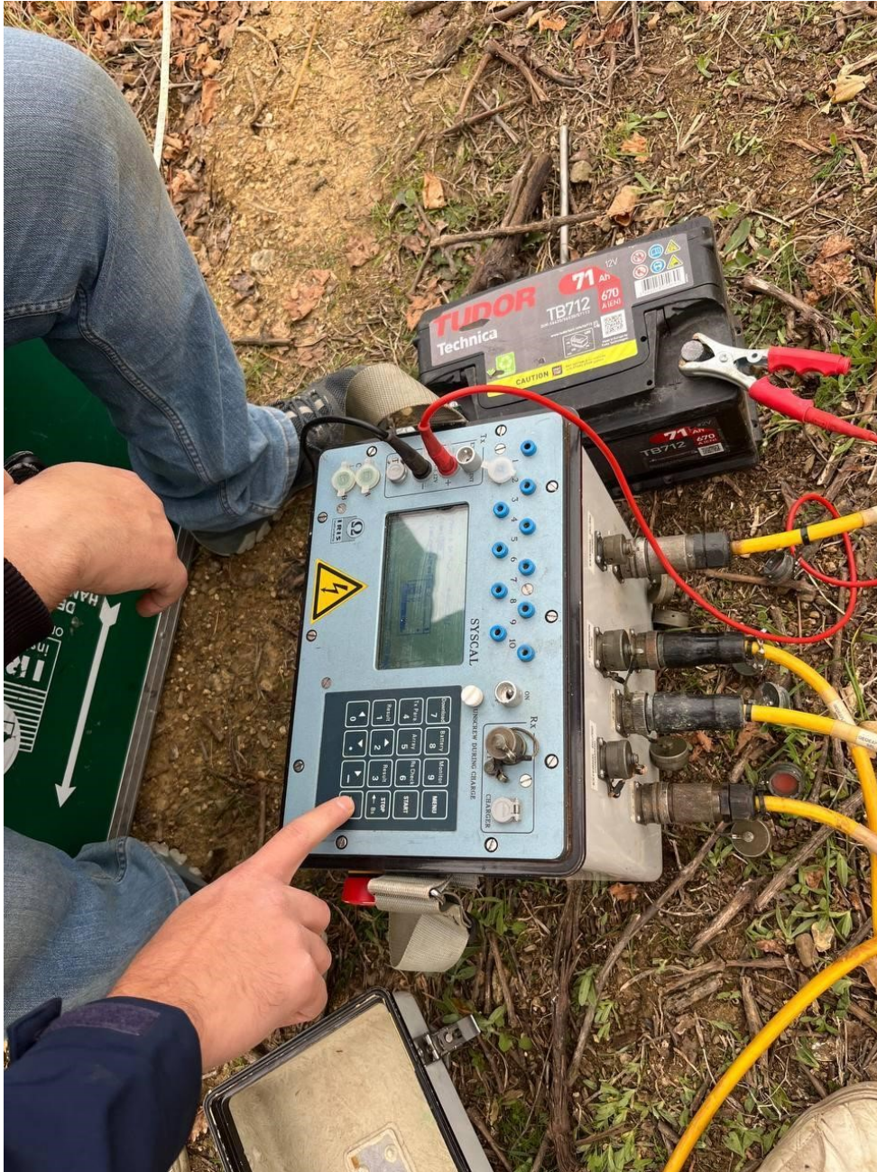
Figure 6.5. 3D ERT Data acquisition with syscal pro georesistivitymeter
