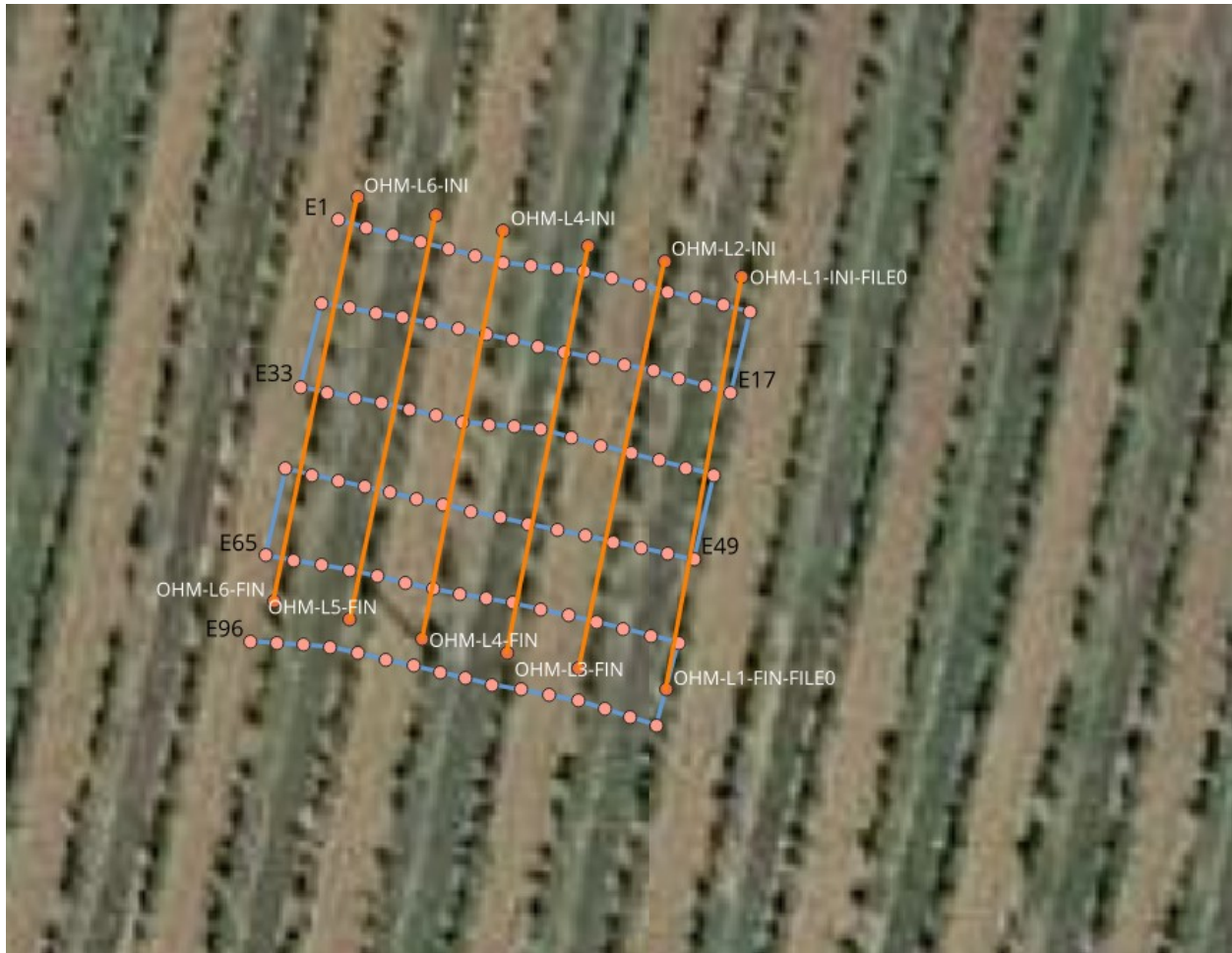
Figure 6.2. GPS Electrodes position in 3D ERT measurement and also 6 lines of ohm mapper which is perpendicular to 3D ERT measurement with QGIS software
