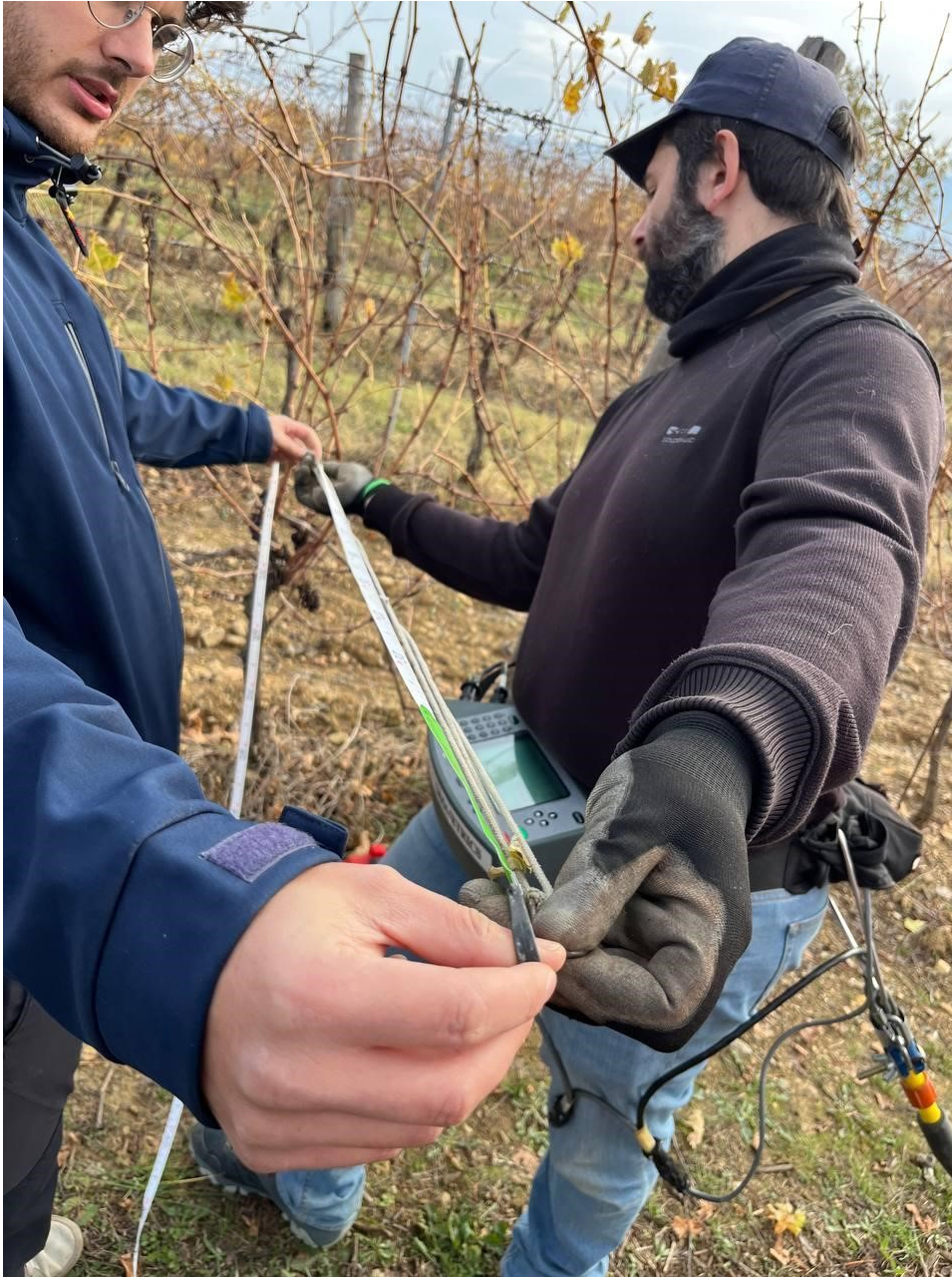
Figure 6.10. non-conductive rope in ohm mapper measurement.
