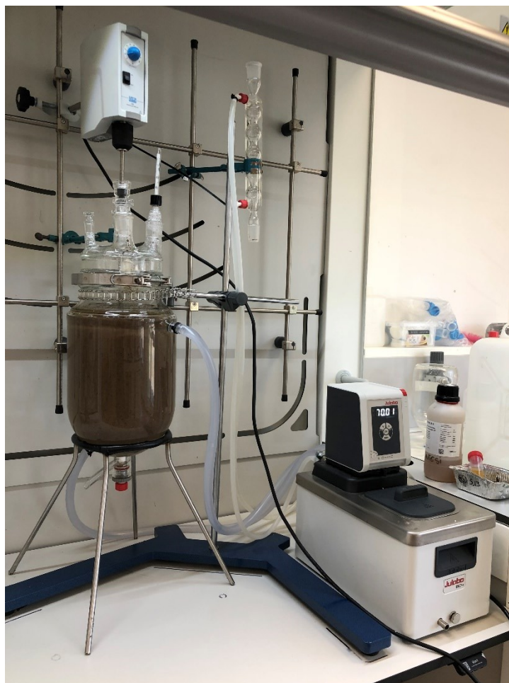
Figure 2.5: Complete apparatus for carrying out the hydrolysis reaction
