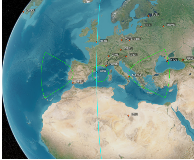
Figure 3.19: Station visibility simulation in MATLAB environment, CCR FOV projection is shown in green.
