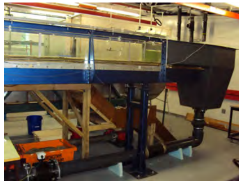
(b) Upstream header tank.
