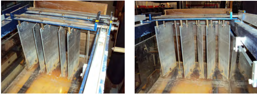
Figure 21: System of floodgates seated at the end of the flume.
