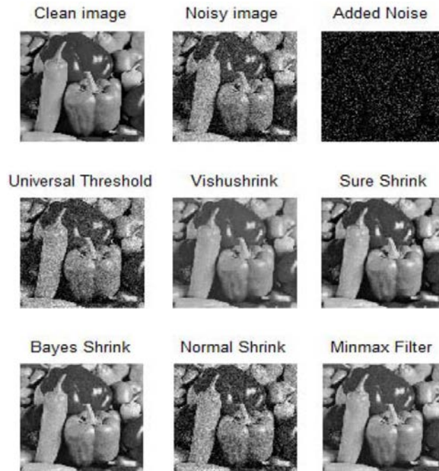
Figure 5-26 Example of filters application on a Smooth Image (Peppers)
