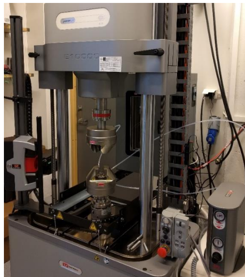
Figure 8-4 Instron ElectroPlus E10000 Fatigue and Static Testing Machine
