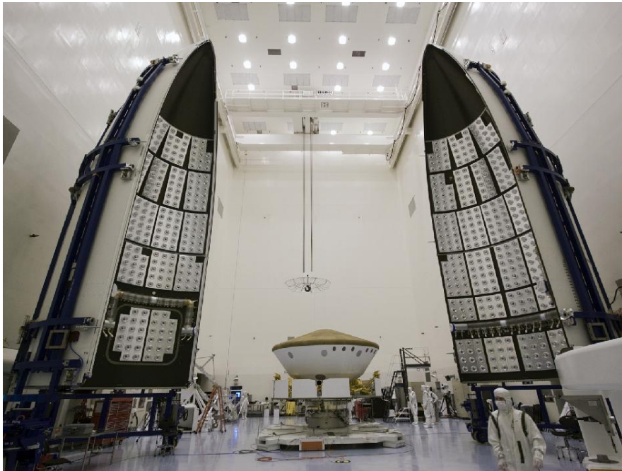
Figure 5.2. A fairing of a launcher system. Image source: [10]
