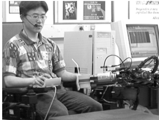
Figure 1.10 – KARES workstation is intended to help users in tasks such as grasping objects and turning off and on light switches.
