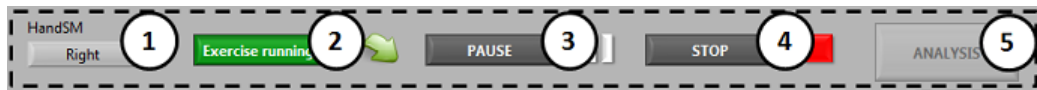
Figure 3.3 – Command panel. 1) Left or right hand option; 2) "Start" button; 3) "Pause" button; 4) "Stop" button; 5) "Analysis" button.
