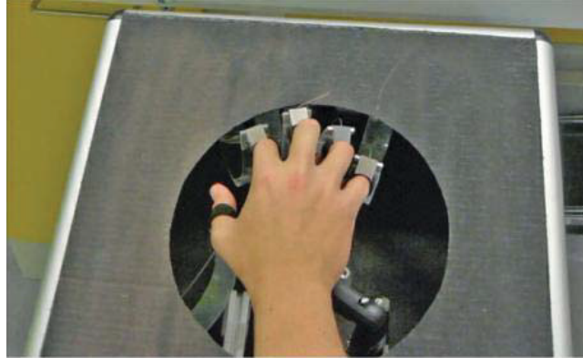
Figure 1.6 – HandCARE3 system. Cables attached to the fingertips can pull the digits open.
