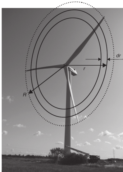
Figure 3.7: Sketch of the division of a wind turbine rotor into annular elements, from (Bak 2013) (Source: NM80 photo at Tjæreborg Enge, Denmark by Christian Bak, DTU Wind Energy.)
