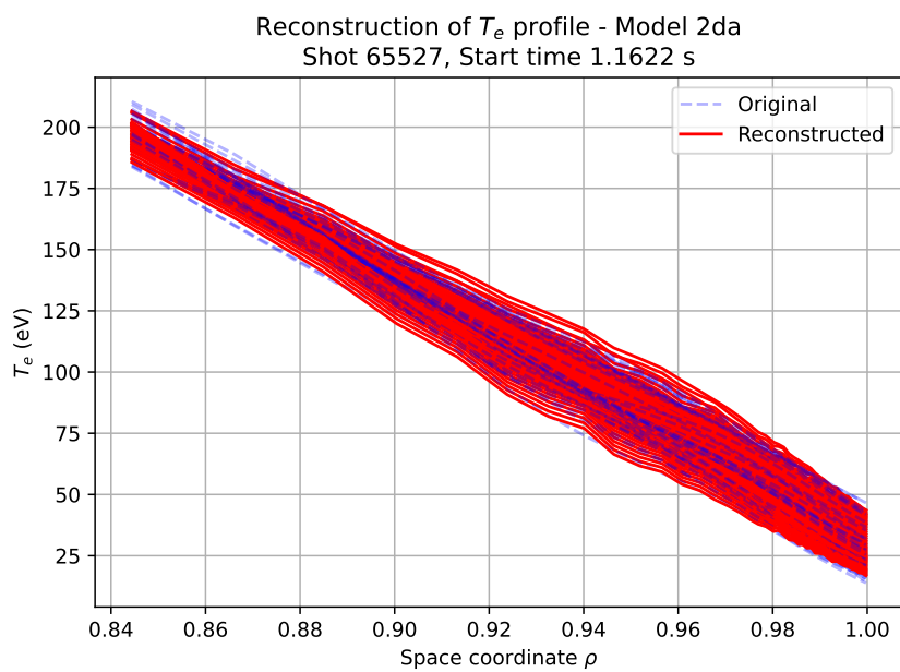
Figure 7.30: Original and reconstructed profile for shot 65527, start time 1.1622s, model 2F.
