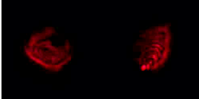
Figure 4.10: Out of focus images of the initial beam. On the left the image after the focus, on the right the image before the focus.
