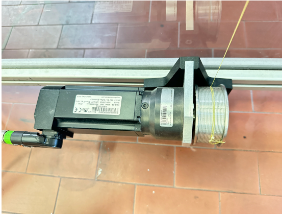
Figure 3.5: Overview of Motor Attached with pulley
