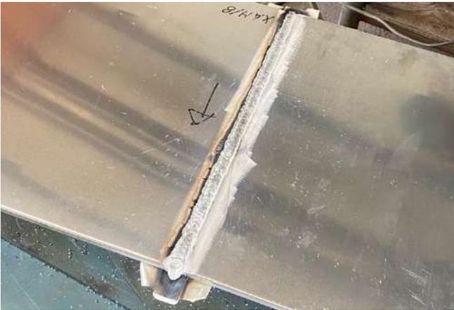
FIGURA 16 SECONDA SALDATURA A MIG
