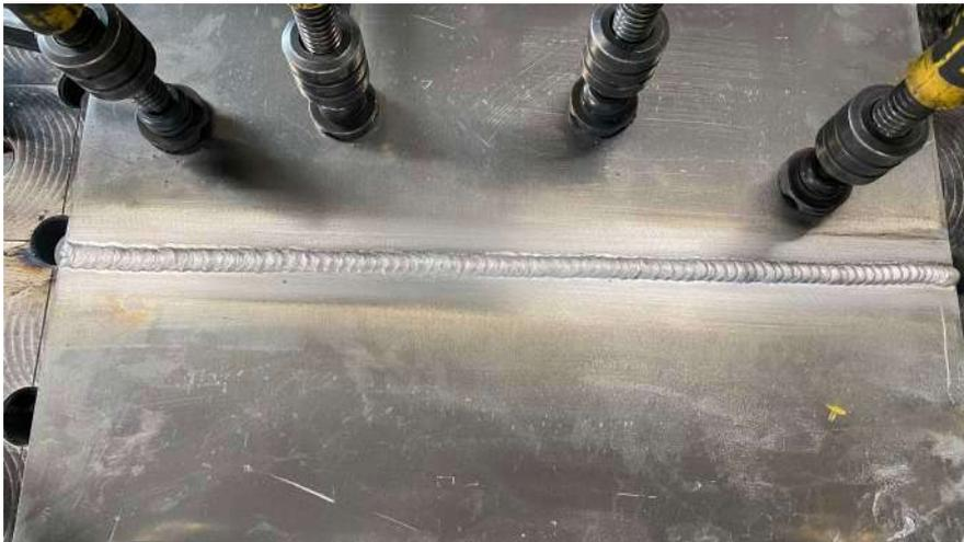
FIGURA 15 SALDATURA A MIG
