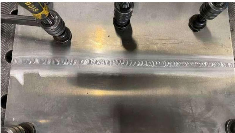
FIGURA 13 SALDATURA A TIG
