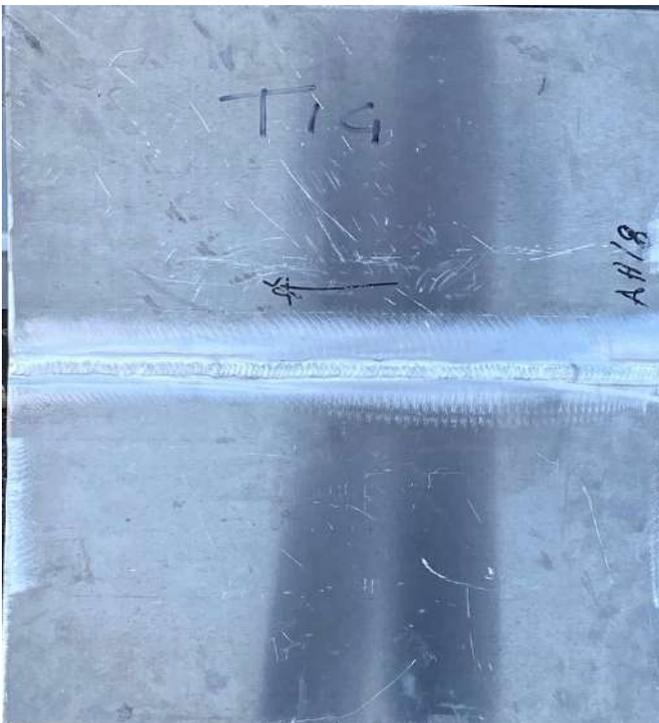
FIGURA 14 SECONDA SALDATURA A TIG
