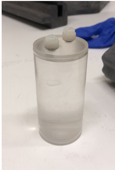
Figure 4.14: Uniform phantom used for calibration.
