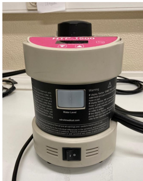
Figure 4.13: Heat therapy pump used to warm up the animal during the scan.
