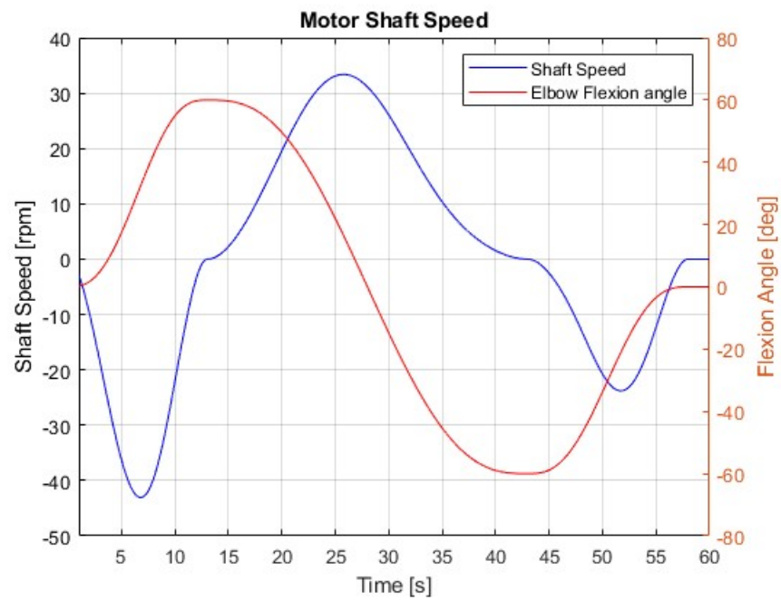
Figure 4.8: Shaft speed ( \omega ) during elbow flexion\extension using PID control
