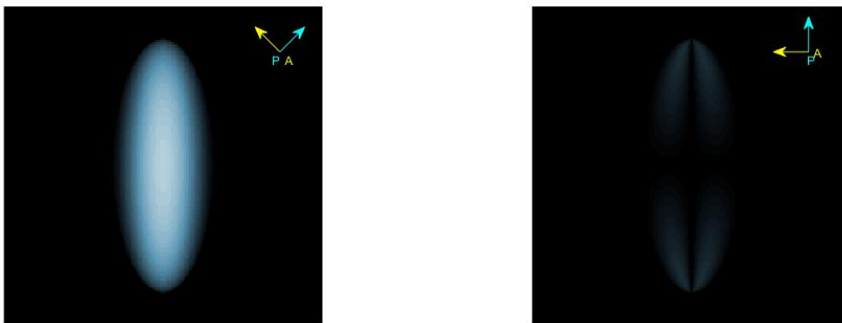
Figure 7.6: Jones matrices simulation for V = 1000 , \alpha = 2.5 , \beta = 1.2 . At two different angles of the polarizers.
