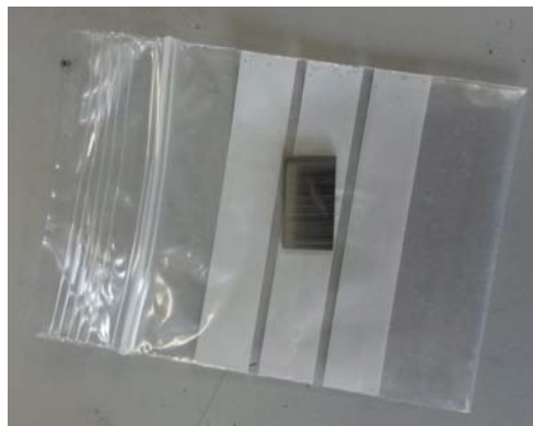
Figure 3.3: Image of a sample after cutting and prior to corners and edges ground.
