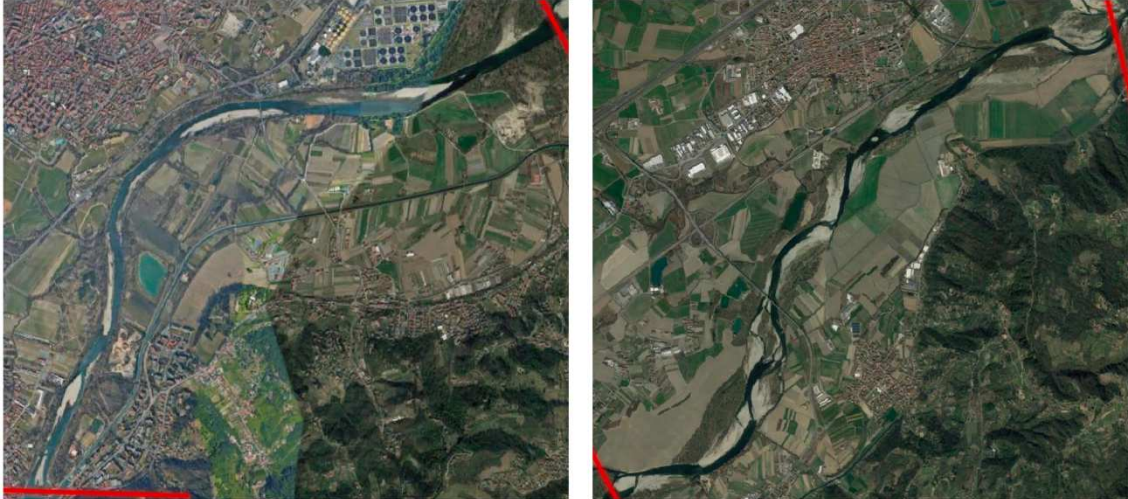
Fig. 20. On the left Po_2, classified as sinuous reach; on the right Po_3 reach, classified as sinuous with alternate bars reach. The red line indicates the starting and ending point found for the identification of the reach.
