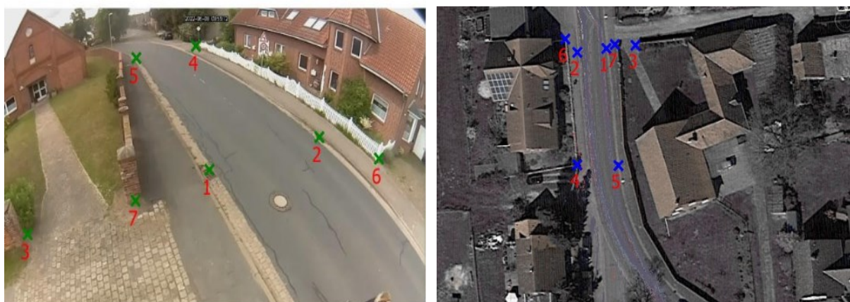
Figure 29 : Homography points in Location 4: camera perspective view and in the 2D in the first picture, aerial view with matching pairs of testers in the right. Source: Mouver-google Maps
