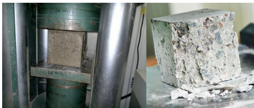
Figure 1.6. Measuring the compressive strength of concrete (Hemali, 2019)
