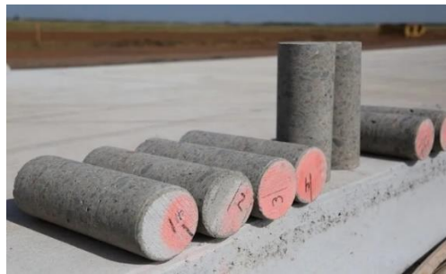
Figure 1.4. Concrete extracted using a cutting machine and concrete sample (Bhushan, 2022)
