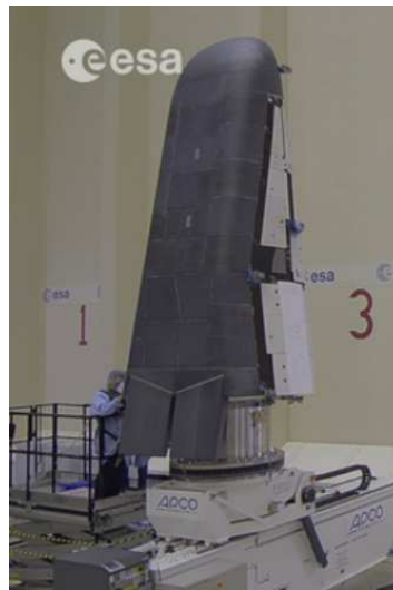
Figure 1.3: IXV vehicle: view of the windward part, from where it is possible to see the two patches of the CATE experiment
