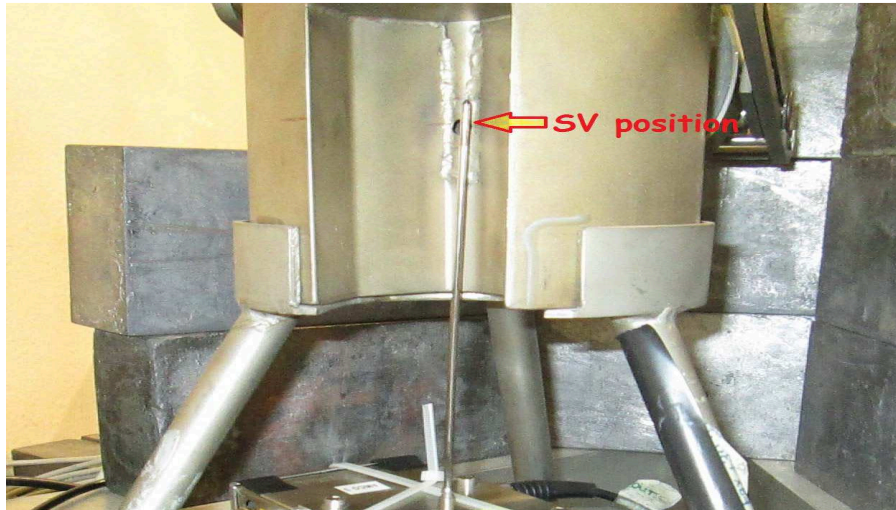
FIGURE 26 – THE GAMMA SOURCE IRRADIATOR AND THE MINI-TEPC. THE GAMMA BEAM EMERGES FROM THE SMALL HOLE BEHIND THE DETECTOR
