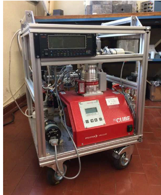
FIGURE 21 - SCHEME OF THE GAS FLOW AND VACUUM STATION AND PHOTO
