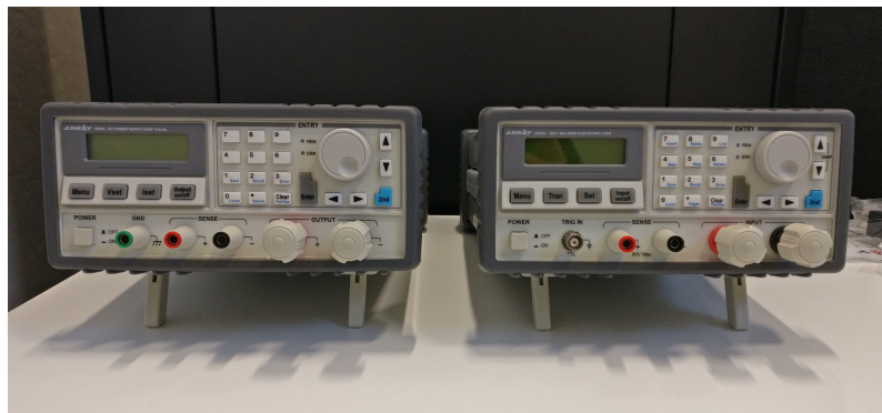
Figure 4.7: Setup instrumentation: Array DC power supply (left) and programmable load (right)
