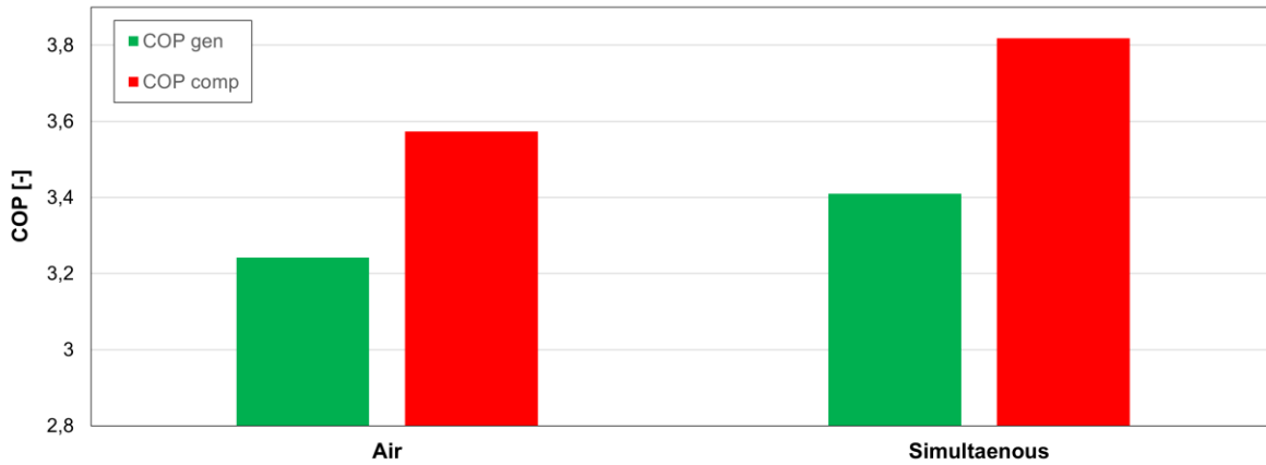
Figure 3.8 – Test performed with G_{TI} = 180 \text{ W/m}^2 , T_{air} = 9 \text{ }^\circ\text{C} , T_{w,in} = 30,5 \text{ }^\circ\text{C}
